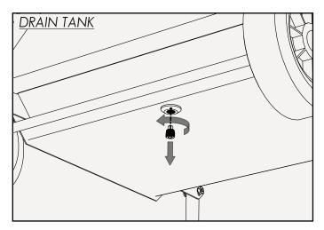
The heater's fuel tank should be drained after each heating season, before long-term storage or transport, or whenever poor fuel quality is suspected. Being careful and prepared to catch and contain the entire contents of the tank, use a 1/4" hex key to remove the drain plug from the tank and allow the contents of the tank to drain completely. Apply fresh thread sealant, replace the drain plug, and confirm that it has sealed properly upon refueling.
