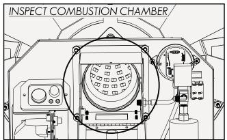
Some visible cracks in the insulation material are normal. If portions of the insulation are broken or missing, replace the insulation before resuming operation of the unit. Contact SunFire technical service for assistance.
