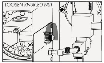
5. Lift the side-retaining plate to rotate it on its hinge. Then, lift the rear of the nozzle subassembly and pull to remove the nozzle subassembly from the burner assembly. With the nozzle subassembly removed, use an inspection mirror to visually inspect the interior of the combustion chamber for signs of fuel buildup or missing portions of the insulation lining.
