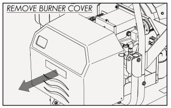
2. Use a Phillips-head screwdriver to remove the screw securing the square access door closed. Then, swing the door down.
