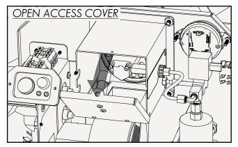
3. Grab and pull the end of the ignition wires (not shown) to disconnect them from the electrode terminals. Then, slide the rubber wire grommets from the housing and move the wires aside.
