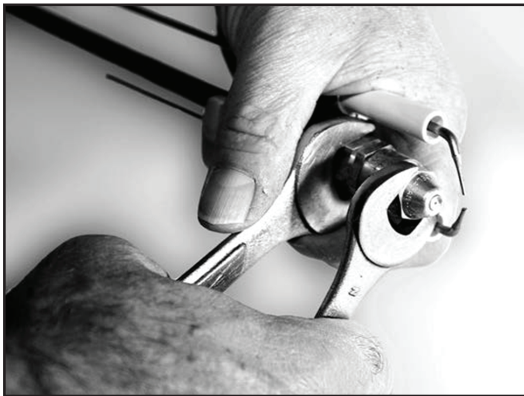
Figure 3A : CAREFULLY SUPPORT THE NOZZLE ADAPTER WHEN REMOVING OR INSTALLING NOZZLE
